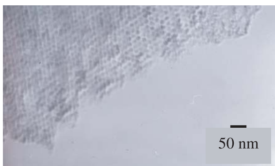
Fig. 1. TEM image of the ordered mesoporous H 1 -platinum phase used in the catalytic reactor study.
